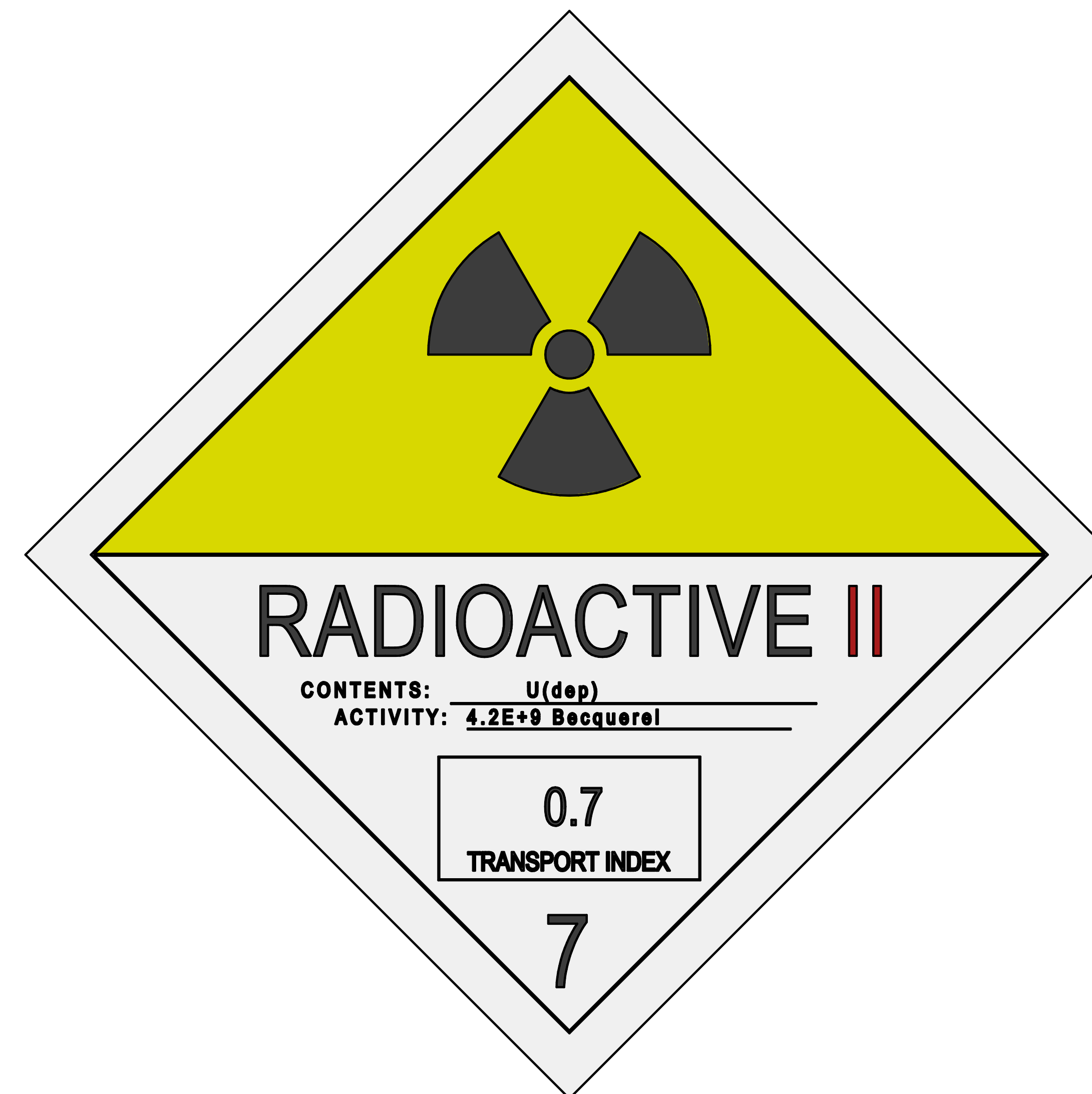
FIGURE 1 DEPLETED URANIUM (DU) LABEL.
