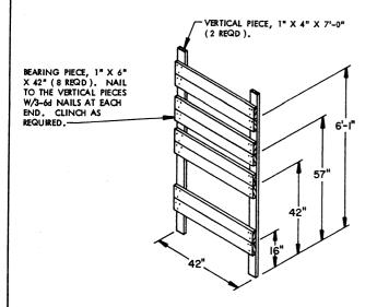
THIS ASSEMBLY IS ONLY REQUIRED WHEN OUTLOADING THE ROUTED DUNNAGE PALLET.
