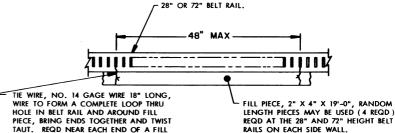
TAUT. REQD NEAR EACH END OF A FILL PIECE AND EVERY 48" OF FILL PIECE LENGTH AS SHOWN.
