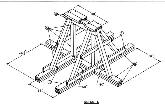
THE OVERALL DIMENSIONS OF THE ABOVE ASSEMBLY ARE 8'-8" LONG X 8'-0" WIDE X 55-1/2" HIGH.
