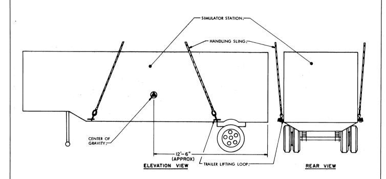
PRECAUTIONARY PROVISIONS FOR HANDLING, STOWAGE AND BRACING AS SPECIFIED IN THE NOTES ON PAGE 2 MUST BE OBSERVED.
