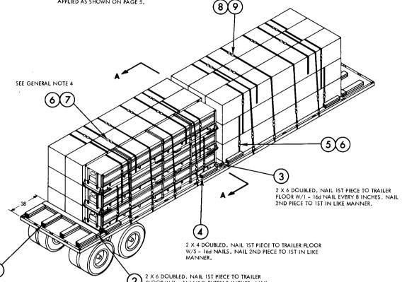
2 X 6 DOUBLED. NAIL 1ST PIECE TO TRAILER FLOOR W/5 - 16d NAILS. NAIL 2ND PIECE TO 1ST IN LIKE MANNER. (BOTH ENDS OF TRAILER.) 2 X 6 DOUBLED. NAIL IST PIECE TO TRAILER FLOOR W/1 - 16d NAIL EVERY 8 INCHES. NAIL 2ND PIECE TO 1ST IN LIKE MANNER. (BOTH ENDS OF TRAILER.)
