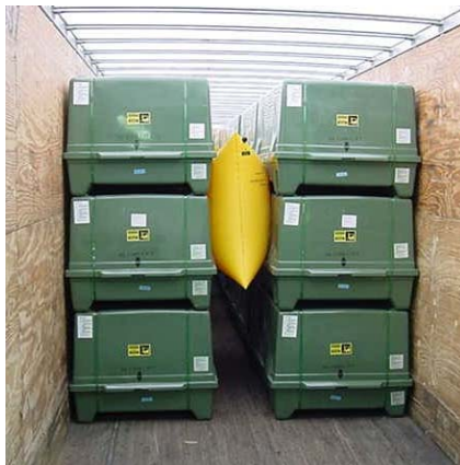
SECTION A-A TYPICAL PLACEMENT OF INFLATABLE BAG
