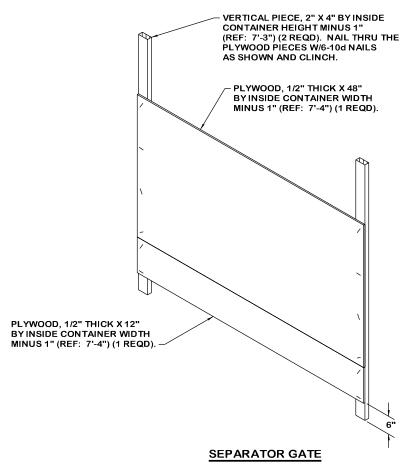
POSITION SEPARATOR GATE BETWEEN THE NOSE END OF THE BOMB PALLETS AND THE CENTER FILL ASSEMBLY IN TWO LOCATIONS AS SHOWN ON PAGE 2. SEE GENERAL NOTES "D" AND "P" ON PAGE 3.
