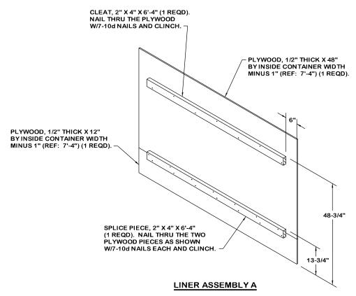
POSITION LINER ASSEMBLY "A" BETWEEN THE BOMB PALLETS AND THE END BLOCKING ASSEMBLY AT EACH END OF THE LOAD AS SHOWN ON PAGE 2. THE CLEAT SHALL BE RECESSED BETWEEN THE RIBS BARS. FIELD CHECK TO INSURE PROPER CLEAT LOCATION. SEE GENERAL NOTES "D" AND "P" ON PAGE 3.
