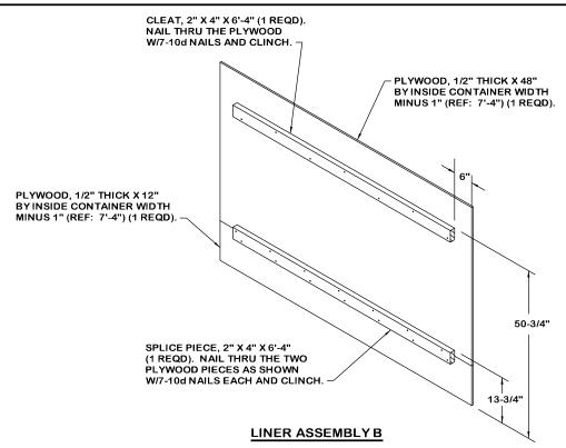
POSITION LINER ASSEMBLY "B" AGAINST THE BASE OF THE BOMB PALLETS AS SHOWN IN THE LOAD ON PAGE 2. THE CLEAT AND SPLICE PIECE SHALL BE RECESSED BETWEEN THE RIBS BARS. FIELD CHECK TO INSURE PROPER CLEAT LOCATION. SEE GENERAL NOTES "D" AND "P" ON PAGE 3.
