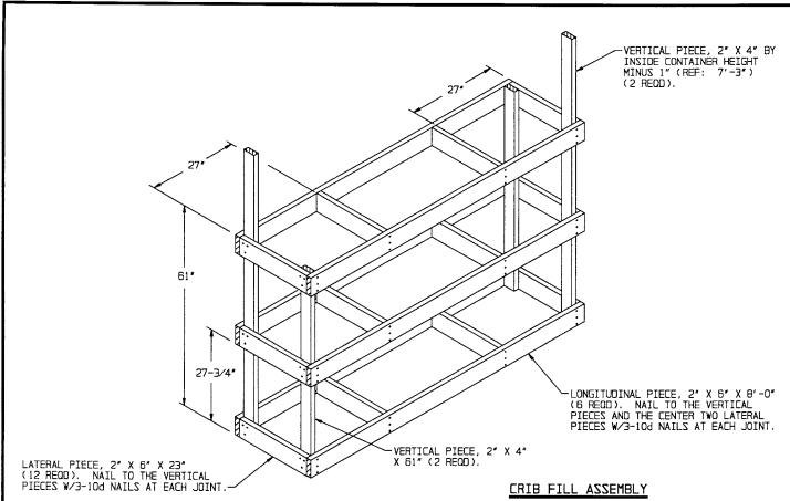
NOTE: FOR A ONE HIGH LOAD, ELIMINATE THE TOP TWO LONGITUDINAL PIECES, AND THE TOP FOUR LATERAL PIECES, AND REPOSITION THE MIDDLE TWO LONGITUDINAL PIECES AND THE MIDDLE FOUR LATERAL PIECES AT 25°, INSTEAD OF 27-3/4°. SHORTEN THE 61° VERTICAL PIECES APPROPRIATELY. THE LENGTH OF THE LATERAL PIECES IS DEPENDENT ON THE VOID BETWEEN THE CNU-554/E CONTAINERS.
