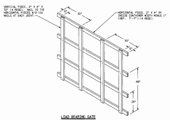
NOTE: FOR A TWO HIGH LOAD, ELIMINATE THE TOP HORI-ZONTAL PIECE, AND FOR A ONE HIGH LOAD, ELIMINATE THE TOP TWO HORIZONTAL PIECES. SHORTEN THE VERTICAL PIECES APPROPRIATELY.
