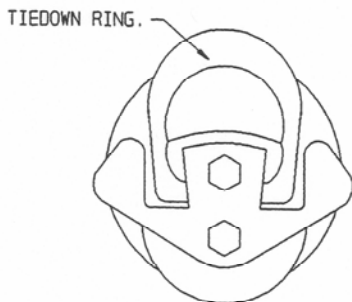
REMOVABLE TIEDOWN ANCHOR (TOP VIEW)
