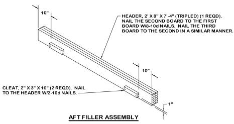
THIS AFT FILLER ASSEMBLY WILL BE PLACED AT THE REAR OF THE LOAD WITH THE CLEATS RECESSED UNDER THE AFT PALLET UNITS. FIELD CHECK IT AGAINST PALLET UNITS TO VERIFY PROPER CLEAT LOCATIONS.
