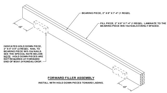
SPECIAL NOTE: HOLD DOWN PIECES (IF REQD) MUST BE RECESSED UNDERNEATH THE PALLET UNITS AND FIT BETWEEN THE PALLET SKIDS. FIELD CHECK DIMENSIONS BEFORE ASSEMBLY TO ENSURE A PROPER FIT. SEE GENERAL NOTES "B" AND "E" ON PAGE 3.
