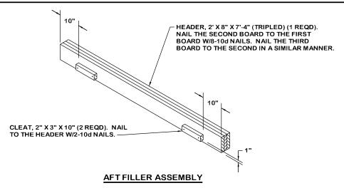
THIS AFT FILLER ASSEMBLY WILL BE PLACED AT THE REAR OF THE LOAD WITH THE CLEATS RECESSED UNDER THE AFT PALLET UNITS. FIELD CHECK IT AGAINST PALLET UNITS TO VERIFY PROPER CLEAT LOCATIONS.
