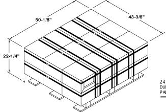
THE LIGHT A064 PALLET UNIT DEPICTED AT LEFT SHOULD BE CONSTRUCTED IAW THE AMC DRAWING LISTED ABOVE WITH THE FOLLOWING CHANGES:
