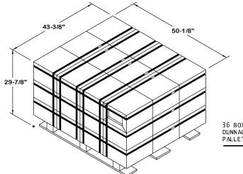
THE LIGHT A064 PALLET UNIT DEPICTED AT LEFT SHOULD BE CONSTRUCTED IAW THE AMC DRAWING LISTED ABOVE WITH THE FOLLOWING CHANGES:
