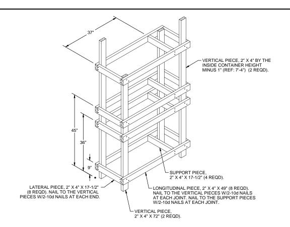
**CRIB FILL ASSEMBLY**FOR A ONE HIGH LOAD, ELIMINATE THE FOUR UPPER LONGITUDINAL AND FOUR UPPER LATERAL PIECES AND ELIMINATE THE TWO UPPER SUPPORT PIECES. REDUCE THE SHORT VERTICAL PIECE TO 36".
