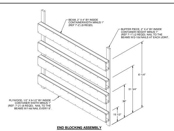
THE DETAIL ABOVE DEPICTS A BLOCKING METHOD TO BE USED WITH A TWO HIGH LOAD. FOR A ONE HIGH LOAD ELIMINATE THE TOP TWO BEAM ASSEMBLIES.
