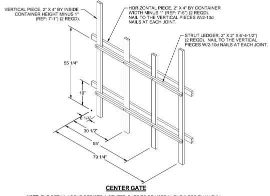
$\underline{\text{NOTE}}$ : THE DETAIL ABOVE DEPICTS A CENTER GATE TO BE USED IN THE "LESS-THAN-FULL LOAD PROCEDURE" DEPICTED ON PAGE 8. FOR A ONE HIGH LOAD, ELIMINATE THE UPPER HORIZONTAL PIECE AND THE UPPER STRUT LEDGER.
