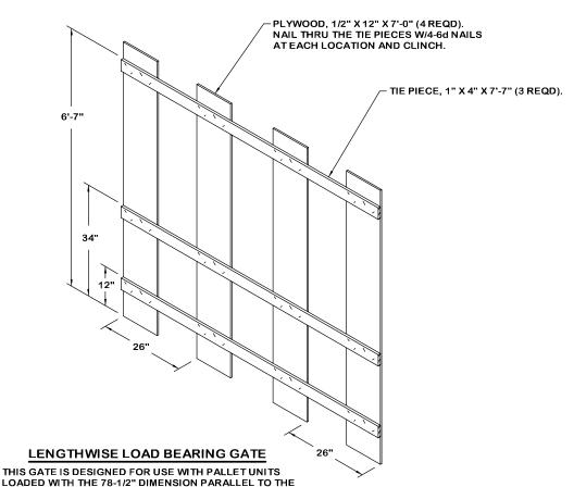
THIS GATE IS DESIGNED FOR USE WITH PALLET UNITS LOADED WITH THE 78-1/2" DIMENSION PARALLEL TO THE LENGTH OF THE ISO CONTAINER. FOR A ONE HIGH LOAD, ELIMINATE THE TOP TIE PIECE AND SHORTEN THE PLYWOOD TO 43".
