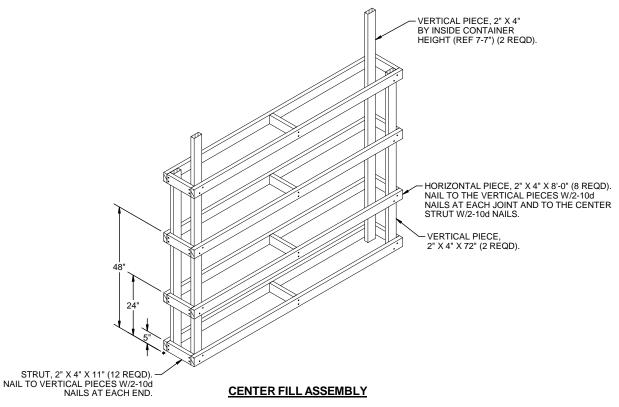
FOR A ONE PALLET UNIT LONG ASSEMBLY, OMIT THE CENTER STRUTS AND REDUCE THE LENGTH OF THE HORIZONTAL PIECES TO 48". FOR A ONE PALLET UNIT HIGH LOAD, OMIT THE TOP TWO ROWS OF STRUTS AND HORIZONTAL PIECES AND SHORTEN THE 72" VERTICAL PIECES TO 24".
