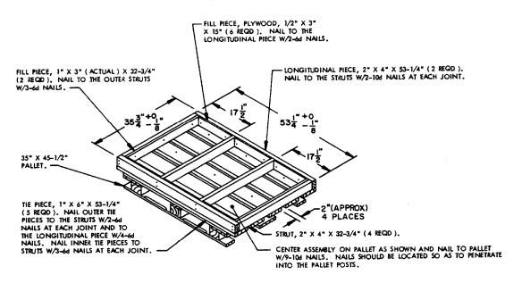
BOTTOM DUNNAGE ASSEMBLY AND INSTALLATION DETAIL
