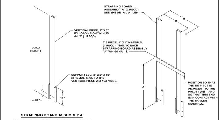
THIS ASSEMBLY IS DESIGNED FOR USE IN THE CHIMNEY PATTERN LOADS SHOWN ON PAGES 10, 16, AND 20.
