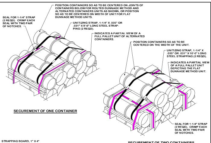
X 22" (2 REQD). INCREASE THE LENGTH OF THE STRAP PING BOARD TO 33" WHEN SECURING FOUR CON-TAINERS.
