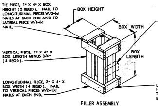
STRAP BEARING PIECE, 2" X 4" X BOX HEIGHT MINUS 3" (AS REQD). NAIL TO VERTICAL PIECES W/2-10d NAILS AT EACH END. NOTE: WHEN A UNIT HAS MORE THAN EIGHT (8) BOXES OMITTED, THE FILLER ASSEMBLY OR ASSEMBLIES LOCATED IN AN OUTER STACK ON THE 42" SIDE OR SIDES OF THE PALLET WILL REQUIRE A "STRAP BEARING PIECE" POSITIONED UNDER THE HORIZONTAL STRAP. STAPLE STRAP TO STRAP BEARING PIECE.
