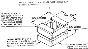
FILL PIECE, 2" X 2" ( RIPPED-TO-FIT ) X BOX LENGTH ( 1 REQD ). - PILL PIECE, 2" X 2" ( KIPPED-IO-PIL ) A BOA LENGTH ( I REQU).
