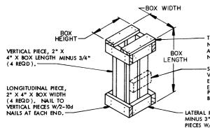
TIE PIECE, I" X 4" X BOX HEIGHT (2 REQD). NAIL TO LONGITUDINAL PIECES W/2-6d NAILS AT EACH END AND TO LATERAL PIECES W/1-6d
