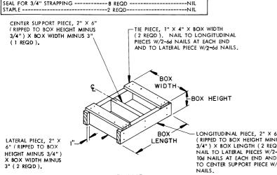
LONGITUDINAL PIECE, 2" X 6" (RIPPED TO BOX HEIGHT MINUS 3/4") X BOX LENGTH (2 REQD). NAIL TO LATERAL PIECES W/2-10d NAILS AT EACH END AND TO CENTER SUPPORT PIECE W/2-10d
