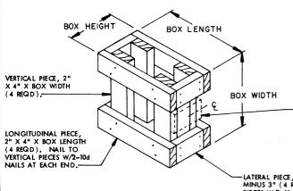
STRAP BEARING PIECE, 1" X 4" X BOX HEIGHT MINUS 3" (AS REQD). NAIL TO VERTICAL PIECES W/2-6d NAILS AT EACH END. NOTE: WHEN A UNIT HAS MORE THAN SIX (6') BOXES OMITTED, THE FILLER. ASSEMBLY OR ASSEMBLIES LOCATED IN AN OUTER STACK ON THE 95" SIDE OR SIDES OF THE PALLET WILL REQUIRE A "STRAP BEARING PIECE" POSITIONED UNDER THE HORIZONTAL STRAP. STAPLE STRAP TO ."STRAP BEARING PIECE".
